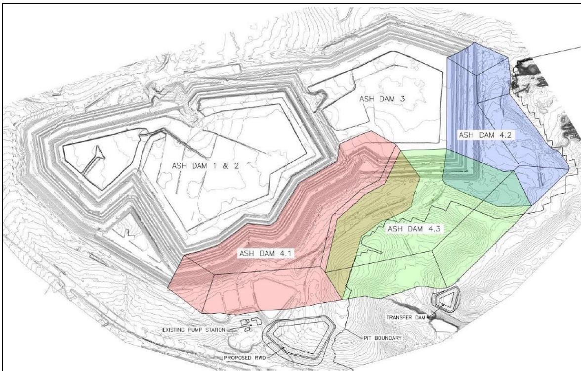
Figure 5 - Ash Dam 4 Concept 2016, consisting of three ash dams (Jones & Wagener, 2016)
