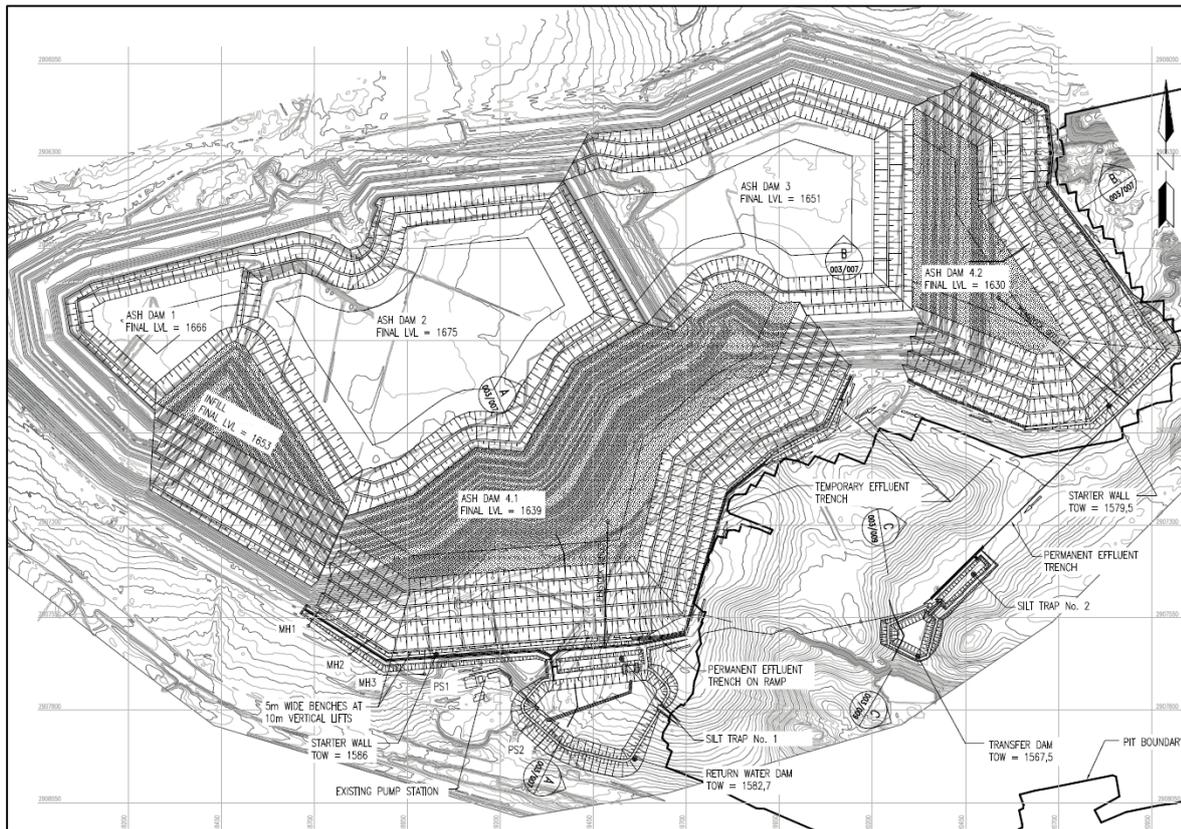
Figure 6 - Ash Dam 4 Concept 2016 preferred alternative, consisting of only AD 4.1 and 4.2 (Jones & Wagener, 2016)
